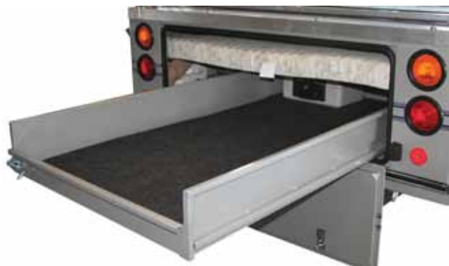
The 280L slide out drawer is accessible through the tailgate when the camper is closed
