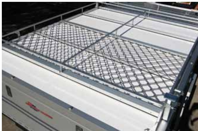
Aluminium mesh on roof rack for extra storage
